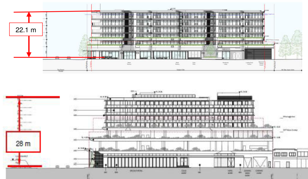
Figure 6: Comparison of the north elevations (Top - updated Sep 2024; Bottom - Design assessed in July 2022)
